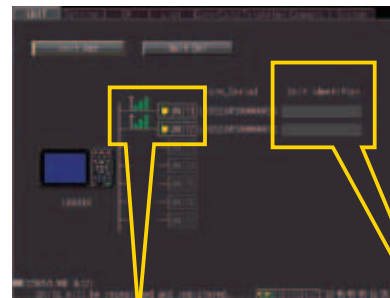
You can verify if the communications state between the LR8410-20 and detected units is good.
