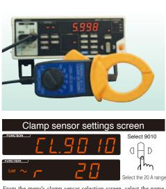
From the menu's clamp sensor selection screen, select the name of the sensor with the cursor key and press the **ENT** key. Then, select the same range as you set for the sensor with the cursor key.
