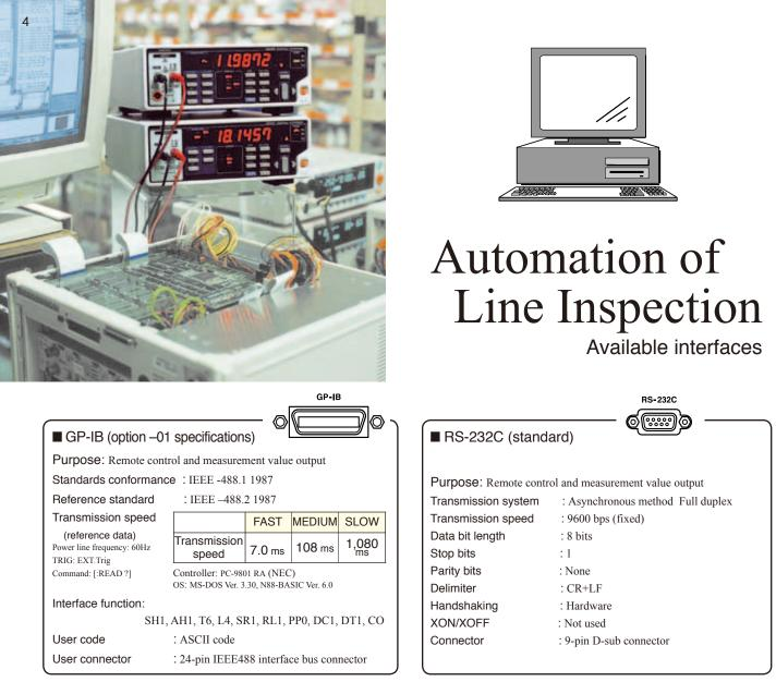
All functions except switching the power on and off can be completely remote controlled and measurement data collected via either the GP-IB or RS-232C interface
