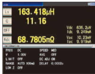
L/Q/ Rdc continuous measurement screen L/Q (1 kHz, 1 mA constant current measurement) and Rdc (DC measurement) display screen
